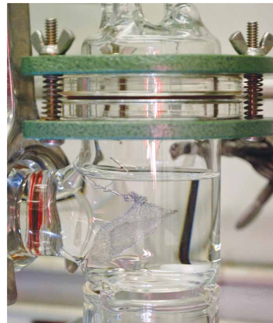
The apparatus used for measuring the electrochemical parameters of the water-splitting reaction. The metallic mesh pictured is a platinum gauze, which serves as an electrode.
