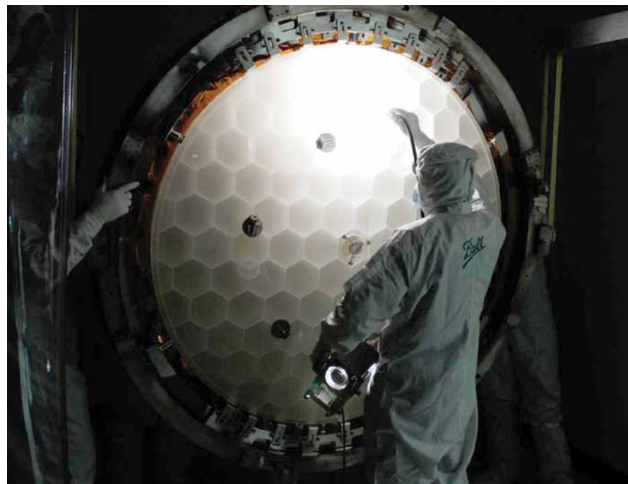
Engineers from Ball Aerospace, the firm that built the Kepler spacecraft, inspect the back side of Kepler’s primary mirror assembly. The mirror is backed by a honeycomb reinforcement structure which is both sturdy and lightweight. You may recognize the Ball logo; Ball Corporation is also one of the largest makers of household glass jars and soda cans!
