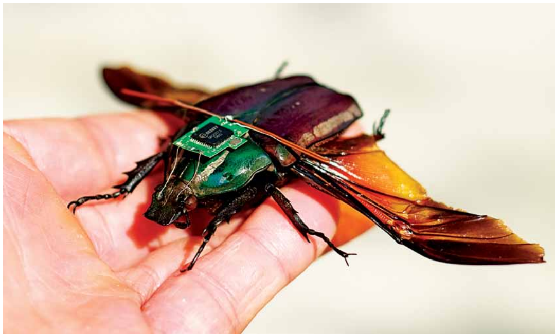
The Mecynorrhina torquata beetle is outfitted with a tiny computer, radio receiver, antenna, and battery. Its asynchronous flight mechanism makes it a good candidate for low-power engineering.
