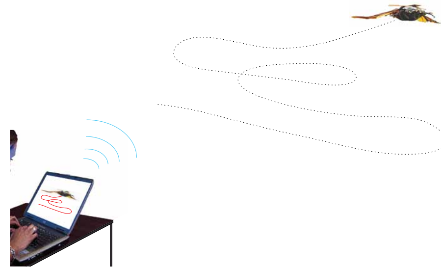
By sending radio signals to circuitry on the beetle, researchers can control the beetle's free flight. Positive and negative pulses to the beetle's brain stimulate the start and stop of flight, respectively, and combining pulses controls flight altitude. Researchers are also able to signal the beetle to turn right or left by stimulating the beetle's basalar wing muscle.
