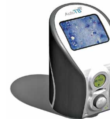
The AutoTB device integrates slide viewing and diagnostic software into a one-step device: users load a sample slide into a slot in the front, and navigate through fields of view on the GPS-like screen.
