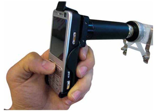
The CellScope fits on the back of a standard cell phone, and uses the phone's built-in camera to capture magnified images of a slide clipped to the end of the CellScope. Software on the phone can analyze the image immediately, or send it via satellite to off-site collaborating doctors.
