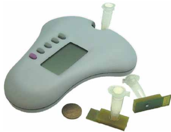
For the home diagnostics market, Silicon Biodevices is testing a hand-held prototype that reads the results of antibody detection from single-use microchips that couple together sample processing and reporting.
